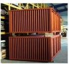
As a heat exchanger surface it uses molded plates stacked into bundles. The plates have gaps between them that make up the space for the air flow. Flue gas flows through the cavities in the plates. This whole assembly is covered with the steel sheathing.
